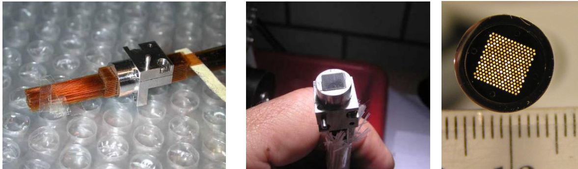
Figure 4: Fiber IFU development. The left panel shows the assembly of the AIP fiber head with a matrix of fused silica capillary tubes clamped in a stainless steel fixture and then filled with fibers. The middle panel shows the same bundle after gluing with Epotek 301-2 low-shrinkage epoxy, cutting and polishing. The head has very small size allowing IFUs to be spaced on the focal surface with a fill-factor as tight as 1/4 . The right hand panel shows the head of the bundle produced by Fibertech, where the fibers were set into drilled stainless steel plates, bonded and polished.
