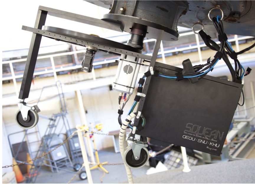
Figure 2. SQUEAN attached to the Cassegrain focus of the 2.1 m telescope. The black box on the right is the electronics box and the small silver one is the CCD camera. The large black disk on the left is the filter wheel. The step motor and the planetary reducer are assembled at the bottom of the filter wheel. (A color version of this figure is available in the online journal.)
