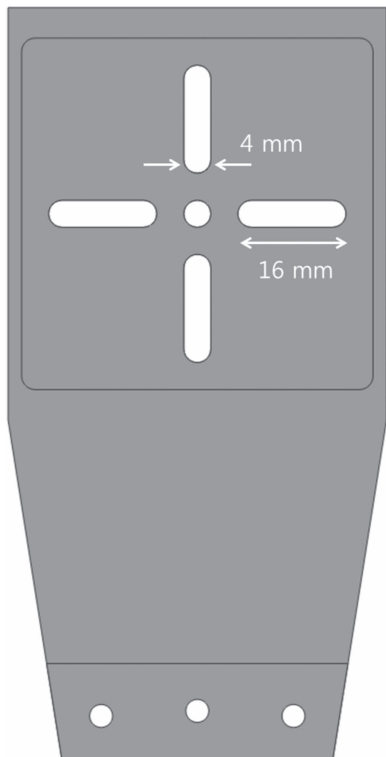
Figure 11. Three-dimensional modeling image of the initial filter mask for filter wheel calibration. This mask can be easily replaced with a science filter during observation.
