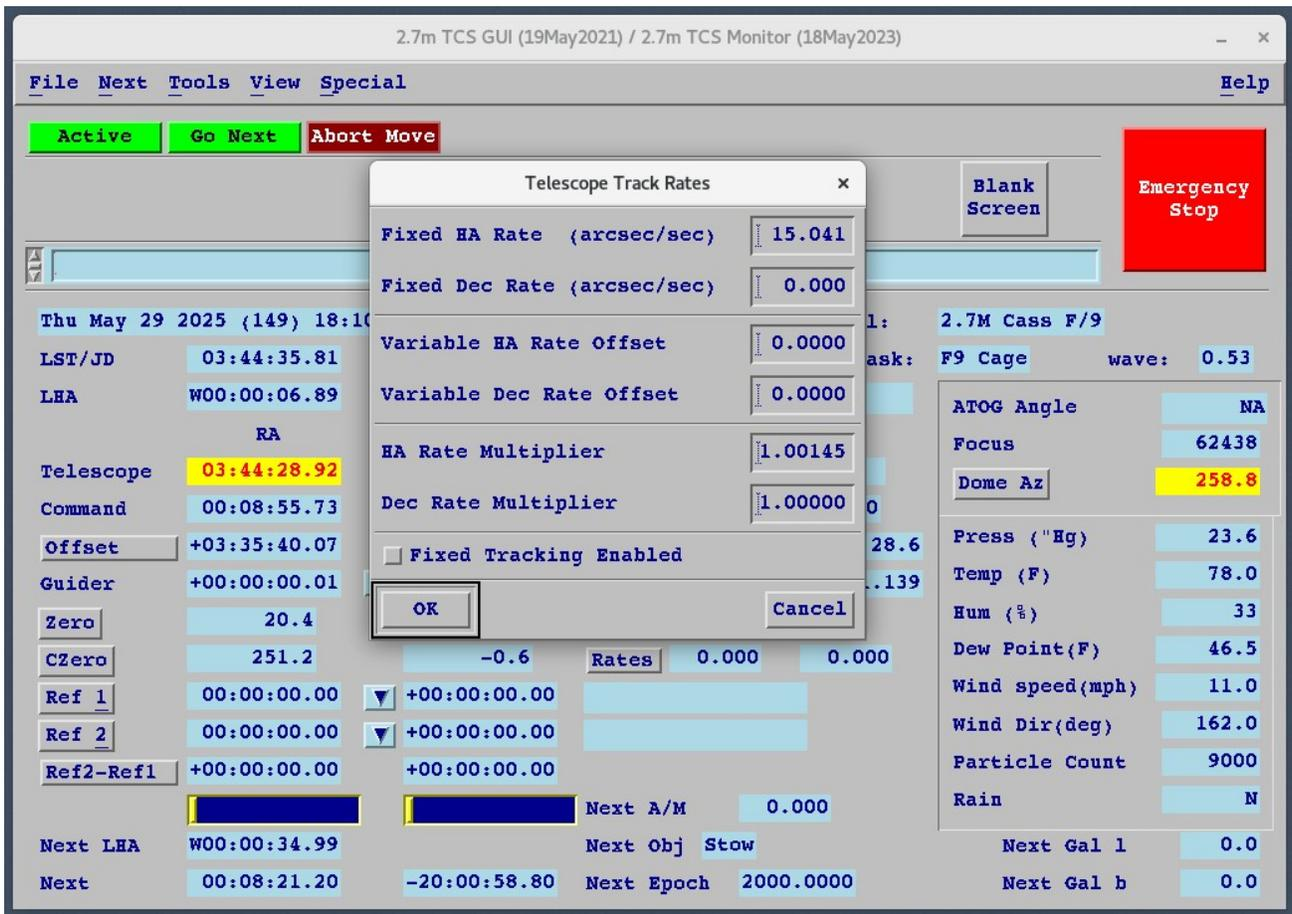
**Figure 8:** The Telescope Control System (TCS) GUI after the *Rates* button has been mouse clicked to popup the *Telescope Track Rates* window. The *HA Rate Multiplier* can be modified to speed up or slow down the telescope tracking. A nominal value is around 1.00130 and the value might range from about 1.00120 to 1.00150
