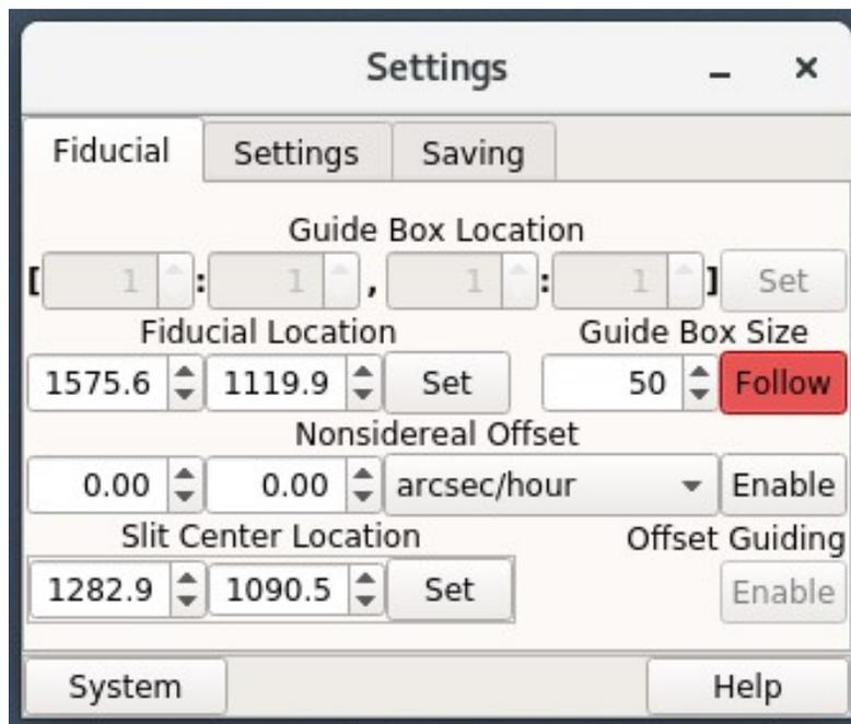
**Figure 4:** The guider *Settings* window, with the 'Fiducial' tab selected. The *Enable* button for Offset Guiding is greyed out (and so cannot be enabled) at this step in the procedure.
