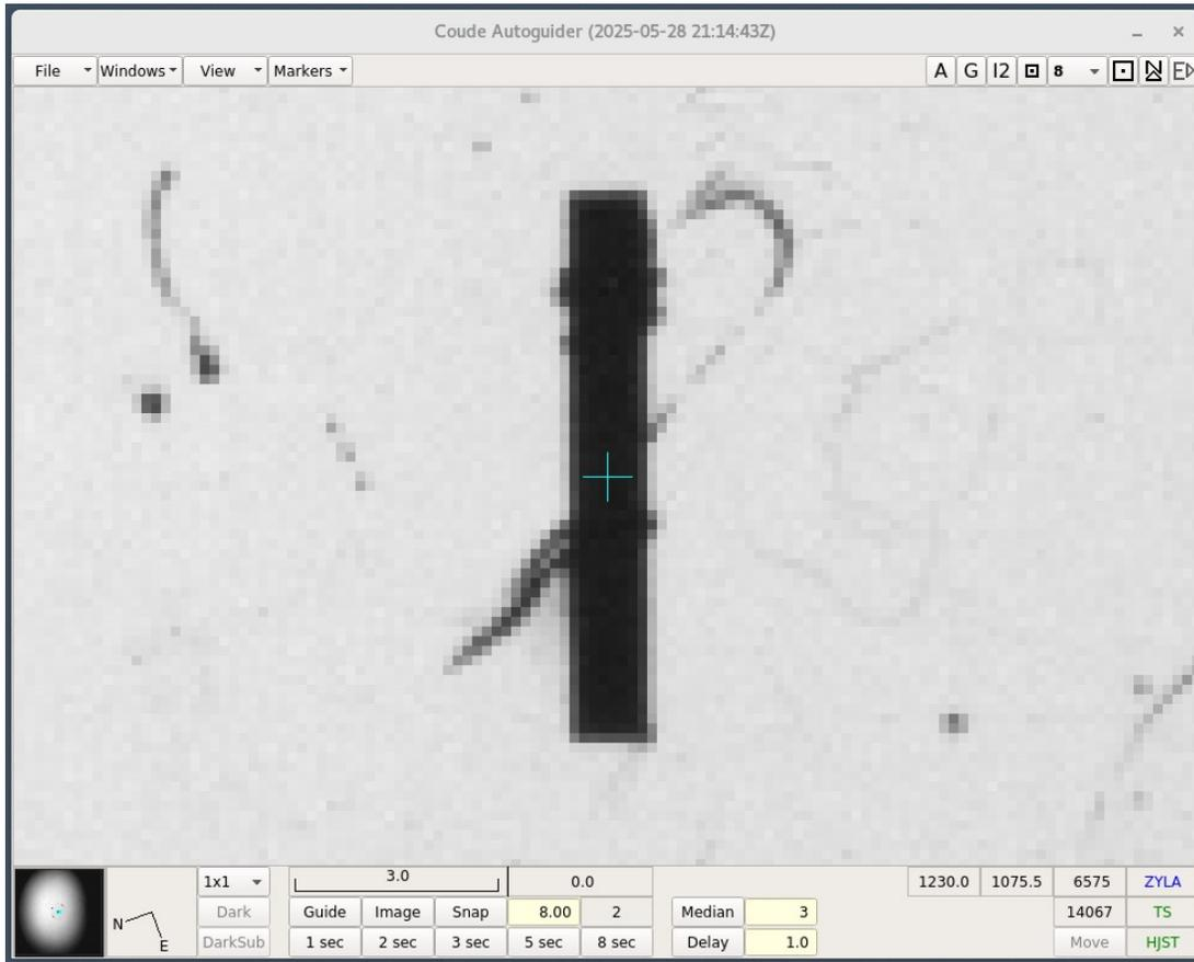
**Figure 3:** A zoomed in image of TS2 slit #4 showing the cyan colored *Slit* marker. The light source used for this image was the ThAr lamp in the calibration system. The various irregular marks around the vertically oriented rectangular slit are scratches due to mishandling of the slit during its lifetime.
