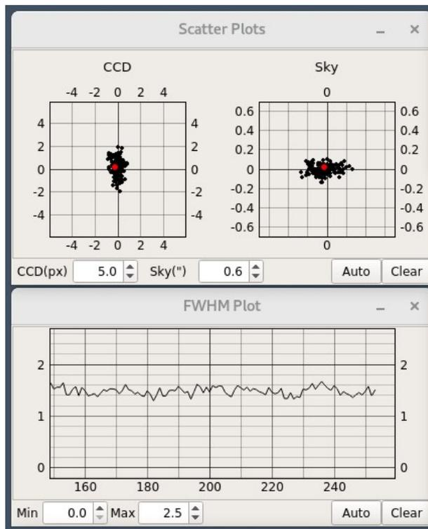
**Figure 7:** Guider *Scatter* and seeing Full Width at Half Maximum (*FWHM*) plots. The scatter plots show the pointing corrections sent to the telescope, with the latest correction shown in red. In the *Sky* plot corrections that move the telescope north are positive, as are corrections that move the telescope east.
