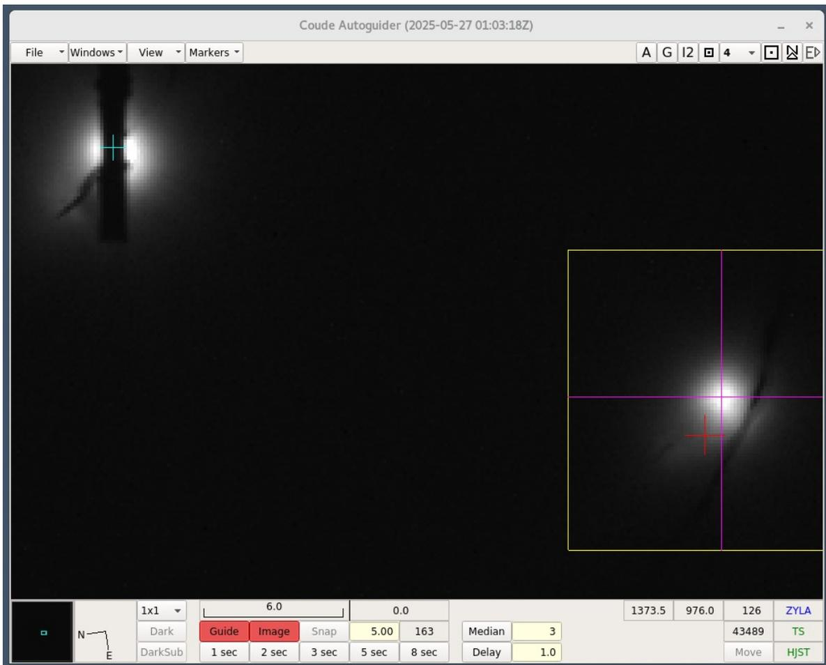
**Figure 1:** A science target star on the center of the spectrograph slit (cyan marker) with a guide star on the guiding fiducial (magenta marker) within the yellow guide box. The guide star was on the red marker when off-axis guiding started.
