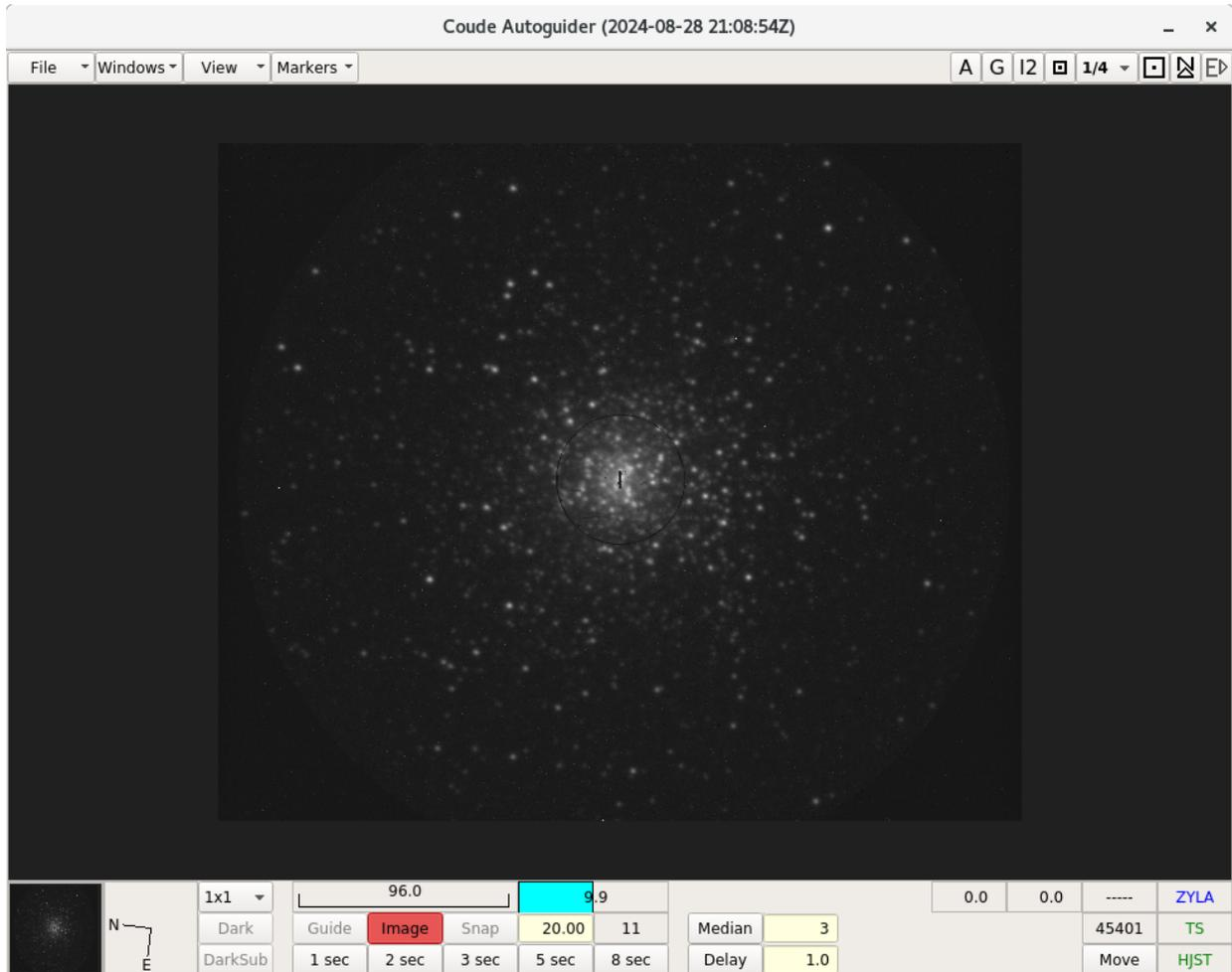
**Figure 2:** a guider image of globular cluster M15. An isolated brighter star in the outer field can be used for off-axis guiding when any particular point such as the black hole location in the cluster core needs to be observed.
