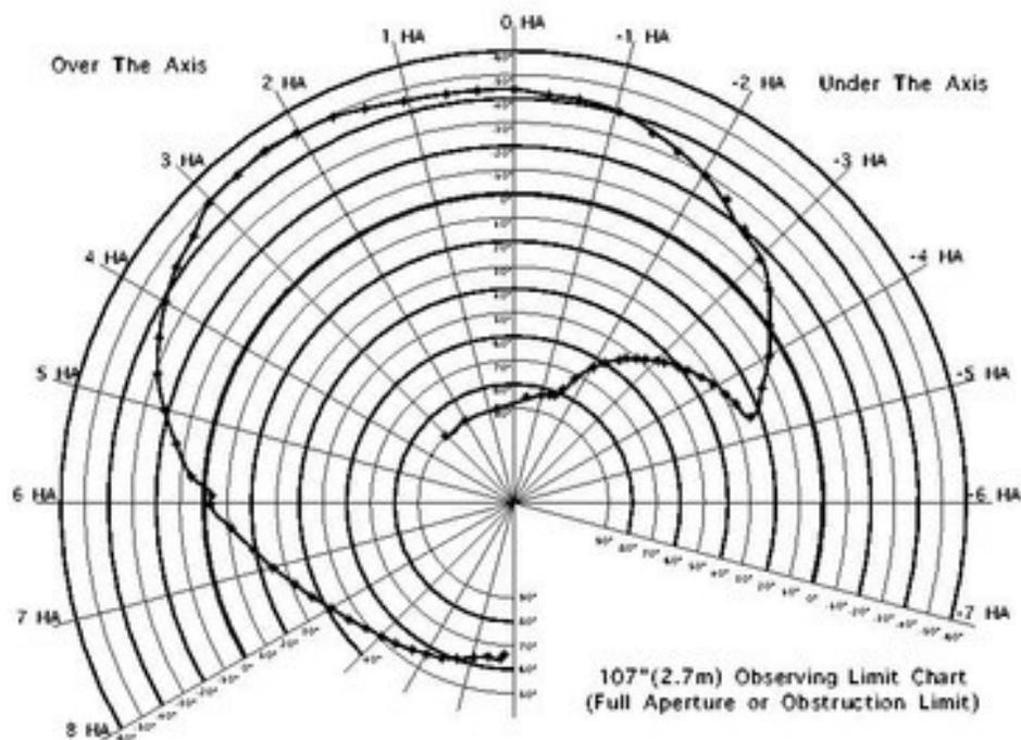
These weights, along with a fairly bulky north pier means that there are regions of the sky that cannot be viewed by the 2.7m telescope. The figure shows the observable limits. Inspection of the figure shows that the observable locations on the sky are a function of both the HA and Declination of the target.
