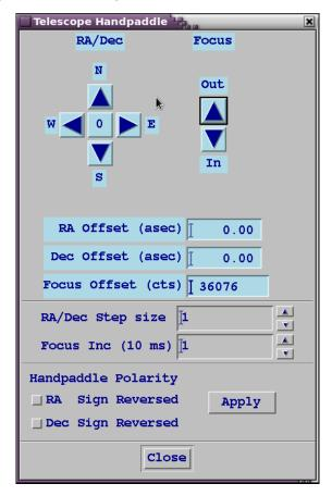
The RA and Dec offset keeps track of manual moves made with the arrows. Clicking on the "0" in the middle of the arrows sets back to the initial position.
