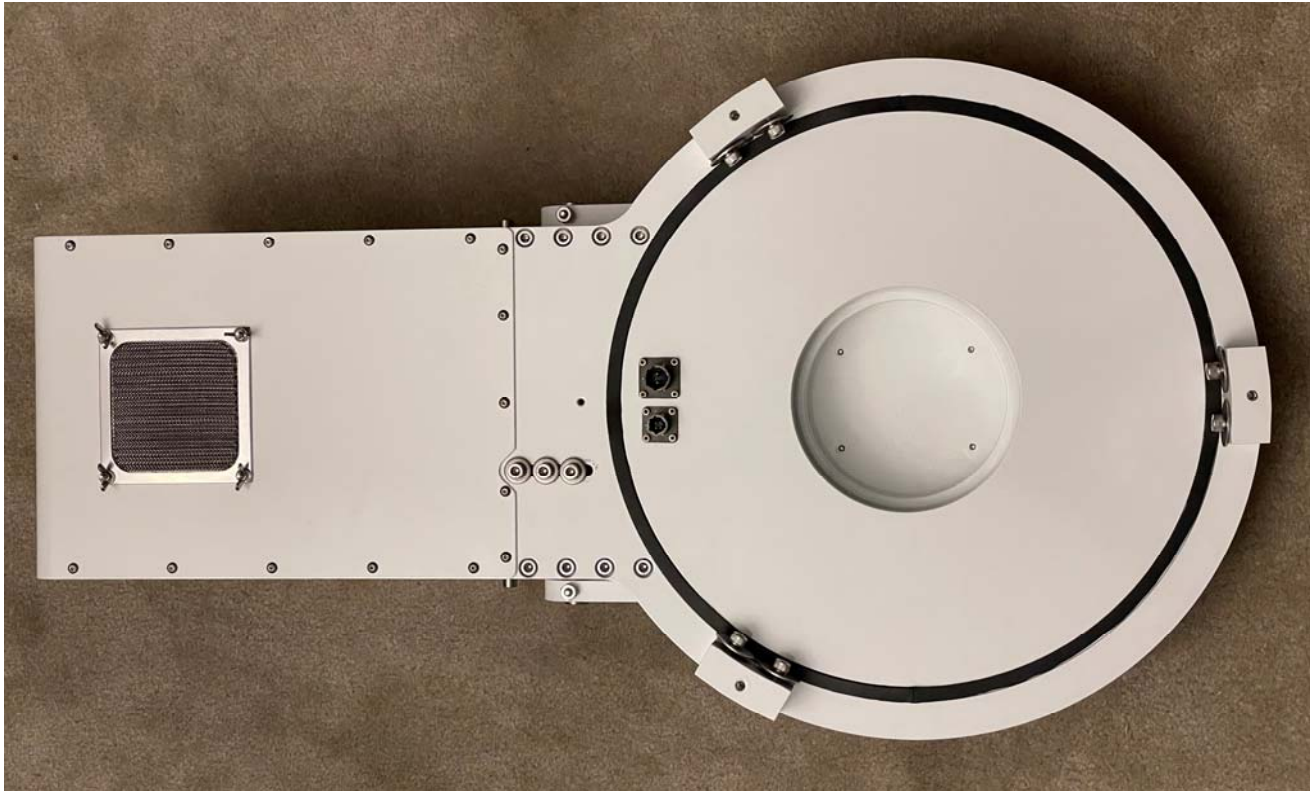
Figure 8: The underside of the Solar Port Cover showing the gasket seated in the gasket groove, the electrical connectors, and a vent into the motor housing.
