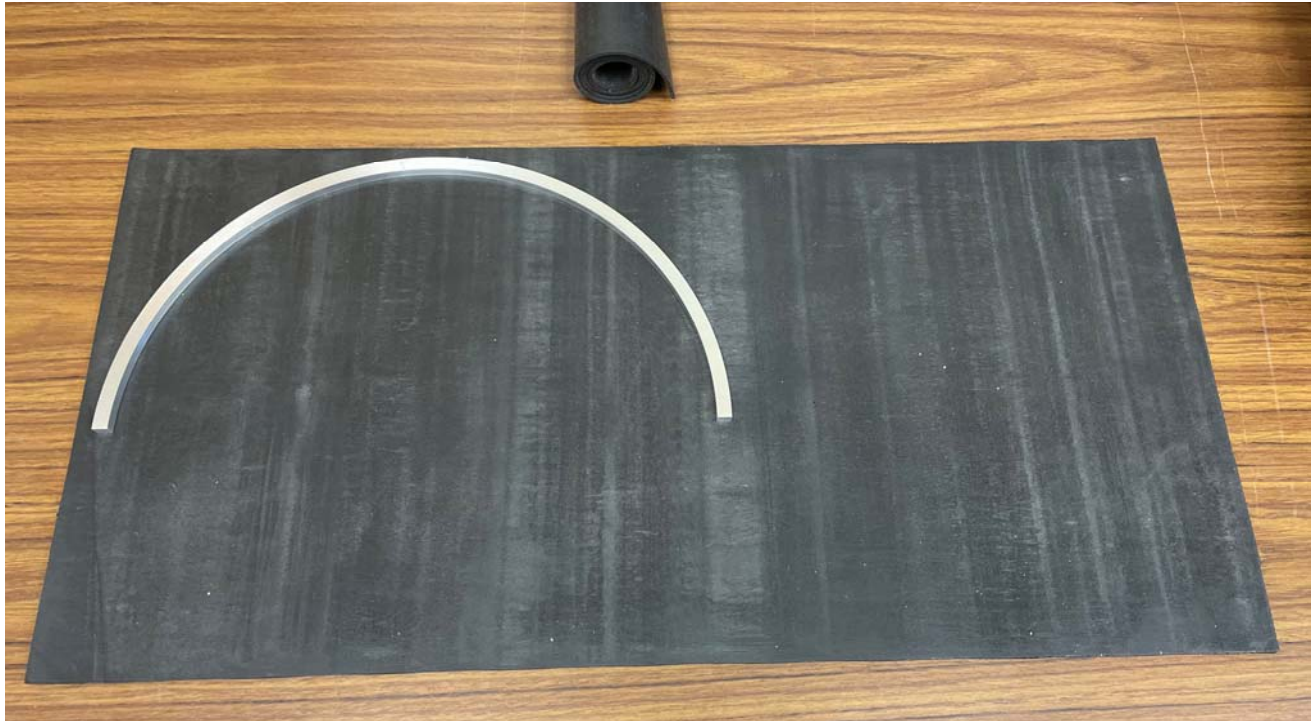
Figure 9: The gasket material and template used in cutting a gasket section.
