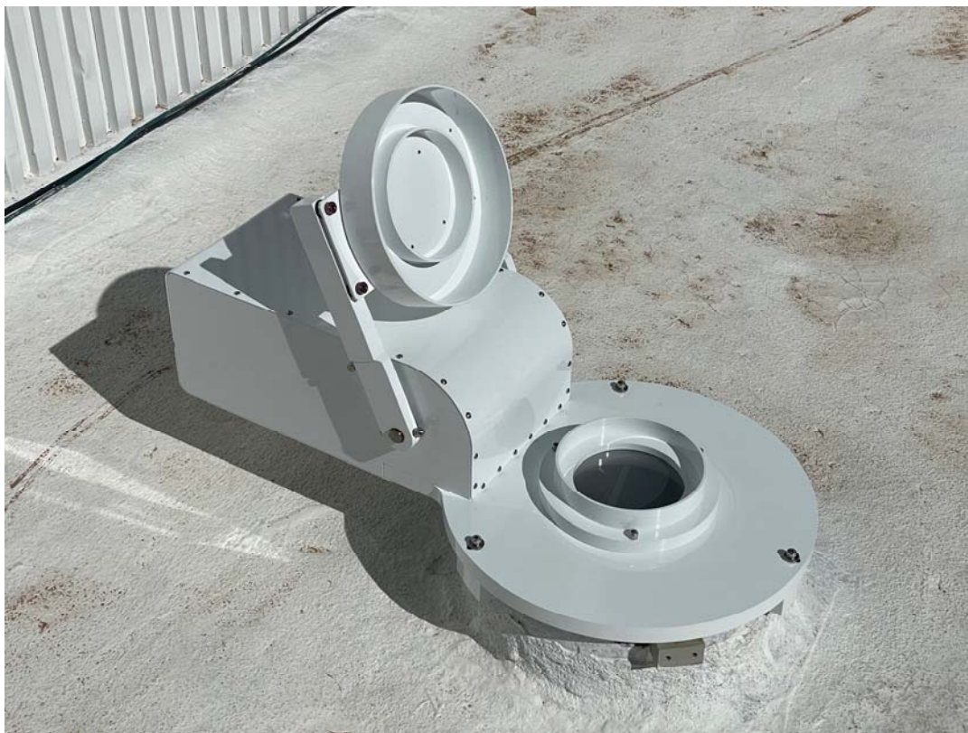
Figure 3: the solar port cover is shown in the open position. The ground glass diffuser optic is seen in the circular opening on the right-hand side. The cover drive shaft is spring loaded when open to prevent cover bounce in the wind.
