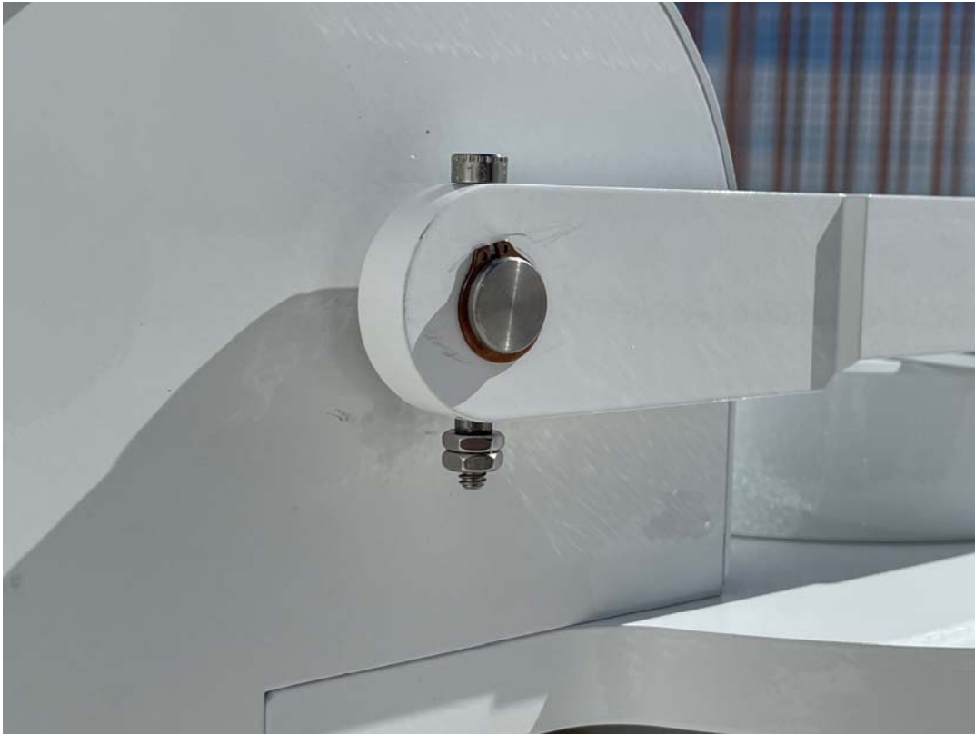
Figure 5: the shoulder bolt and nuts are seen holding one of the cover side arms to the drive shaft. This shoulder bolt is removed on each of the two arms to manually actuate the cover.
