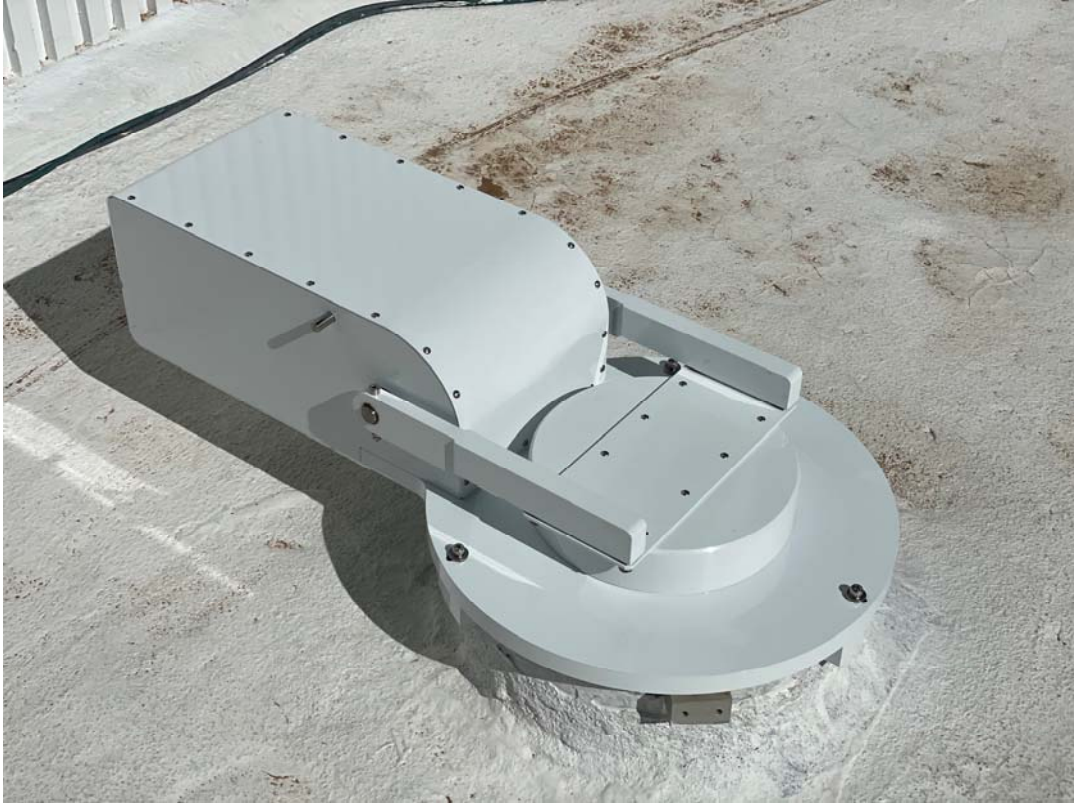
Figure 4: the solar port cover is shown in the closed position. The cover is spring loaded so that it closes flat on the circular base plate, as closing in a cocked position would allow light leakage.
